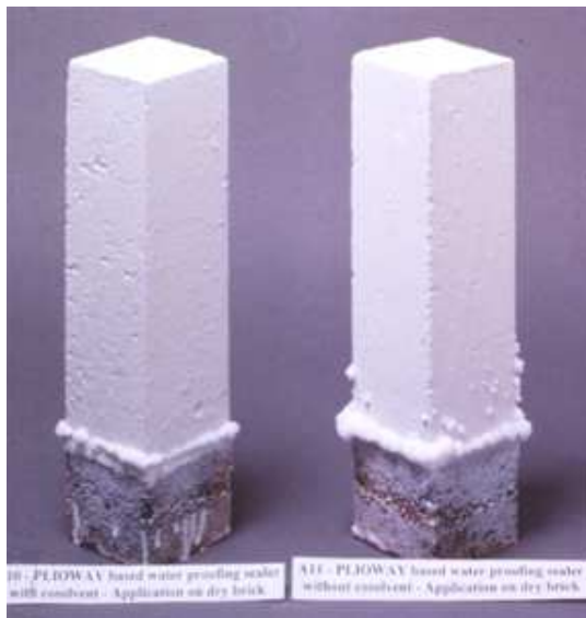
WPS with (left) / without (right) surfactant dry brick
